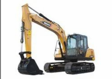
Sany SY140 C-9 14 Ton Crawler Small Excavator
